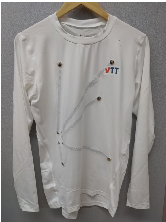
Compression T-shirt with laminated conductive wiring based on stretchable screen printed graphene
